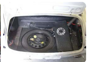
Old versus new. Note the spare tire well sunk into the gas tank.
