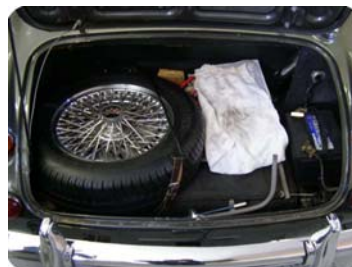
Old versus new. Note the spare tire well sunk into the gas tank.
