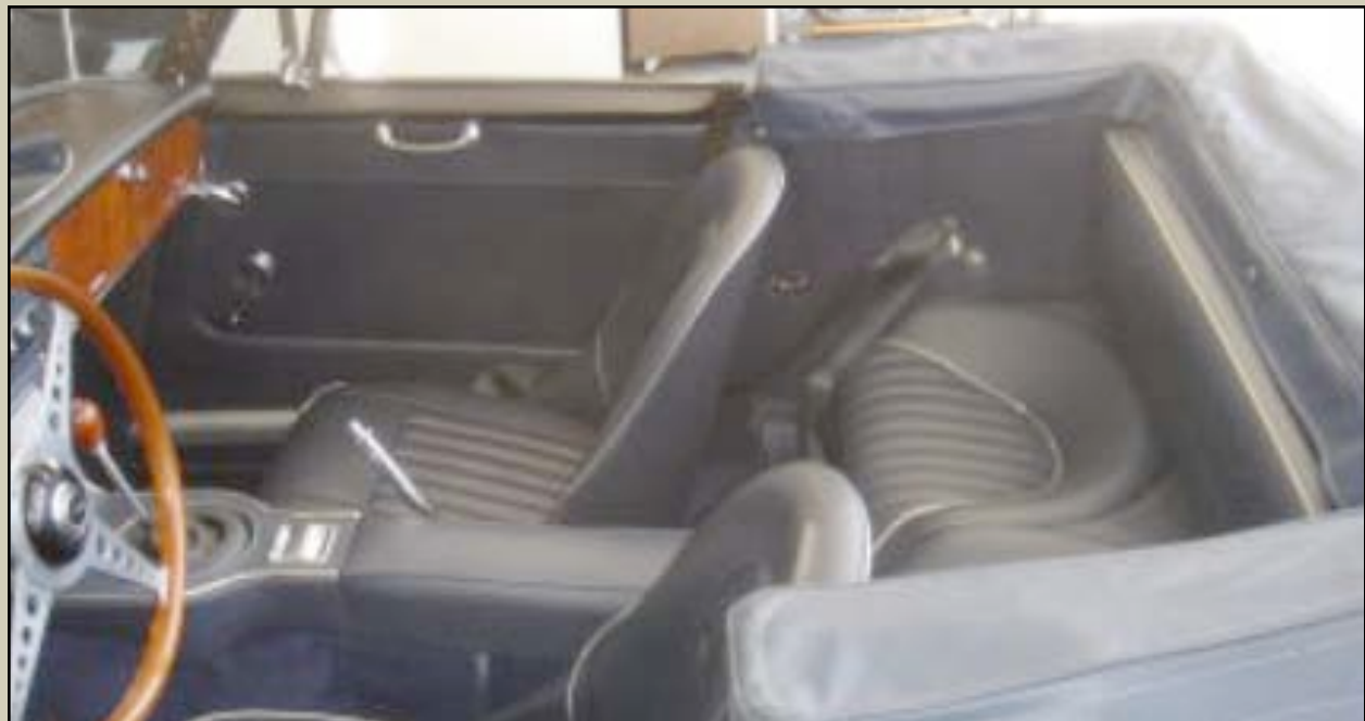
This image shows the added rake angle on the driver's seat back
